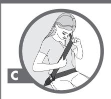
TIGHTEN the lap portion by pulling upward on the shoulder belt. Be sure that the shoulder belt is snug across the chest and crosses the center of the shoulder.
