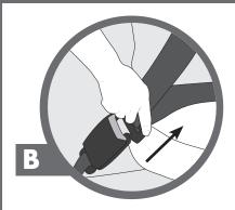
CHECK that the buckle connection is secure by tugging firmly on the seat belt latch plate.
